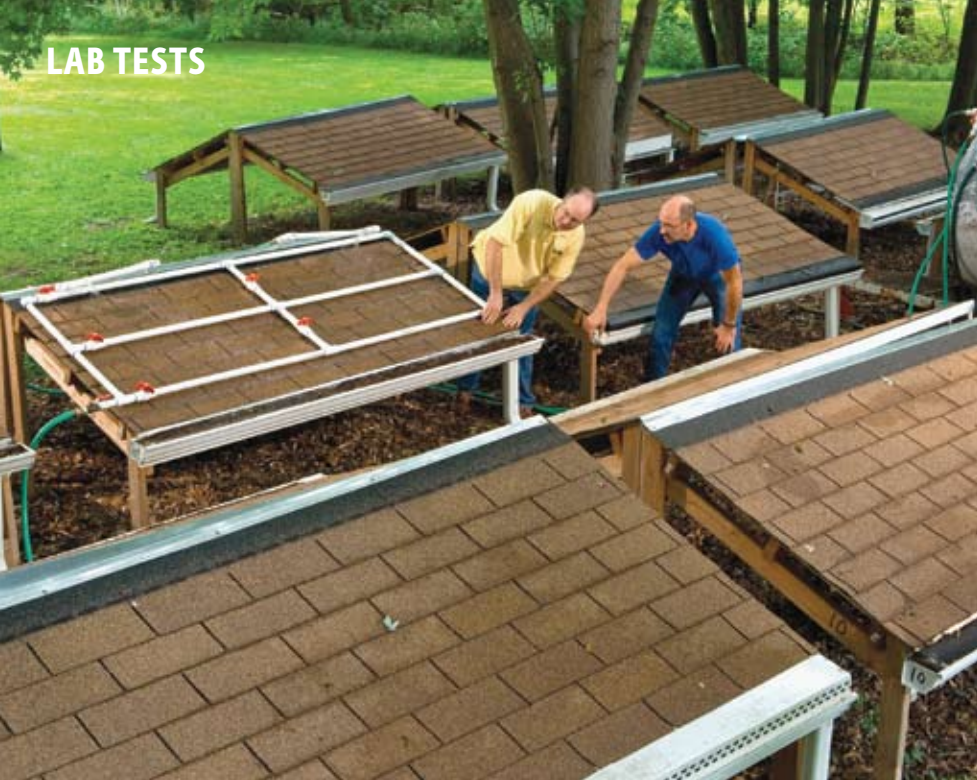
RAINMAKERS Testers simulate rainfall on one of the roof systems built for this report.
