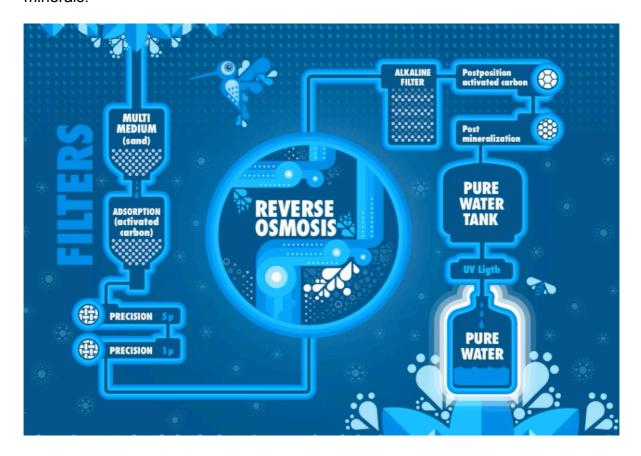
The water firsts arrives at a Multi-medium filter (quartz sand) were the tab water is filter up to 50 microns, removing sediments and particles.
