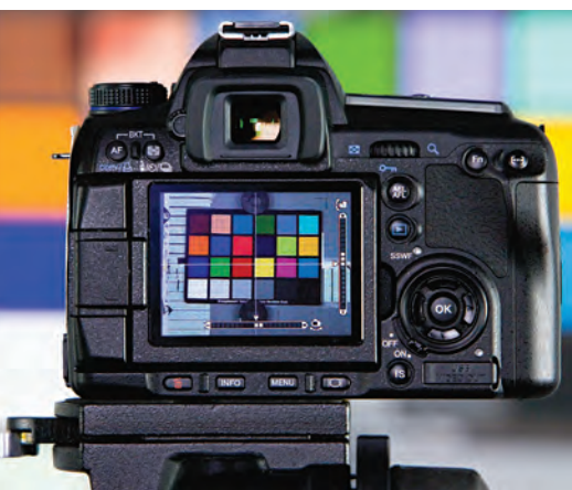
MATCHING COLORS Our camera testers measure how accurately each advanced model captures a set of reference colors.
