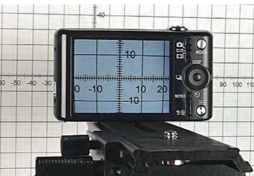
GETTING IT STRAIGHT Each model is tested at various zoom settings to see how faithfully it reproduces a set of geometric patterns.
