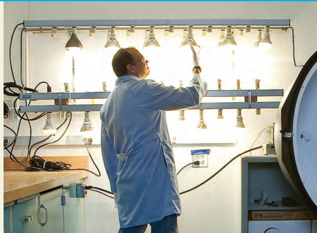
LIGHT YEARS When we tested LEDs to 12,500 hours (about 11 years), most performed as well, or as poorly, as they did after 3,000 hours.
