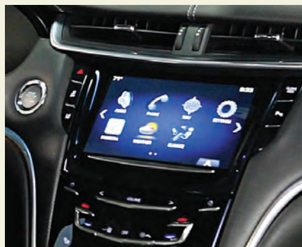
TOUCH INSENSITIVE The XTS's flush capacitive buttons often respond slowly or incorrectly.
