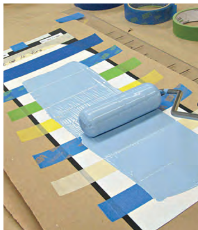
TAPE DECK We tested painter's tapes to see which ones left sharp lines, were easy to remove, and didn't damage surfaces.
