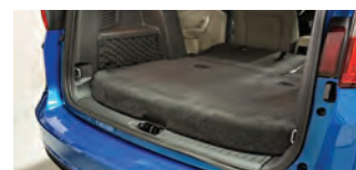
LOAD BUMP The hybrid battery rides under the cargo area, which raises the floor and robs space.
