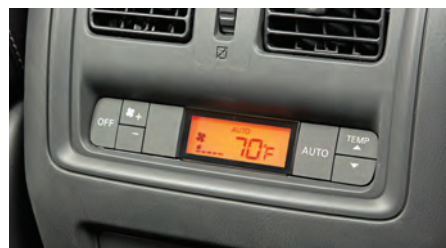
BACK DRAFT The standard three-zone climate system provides basic controls for passengers in the rear seat.
