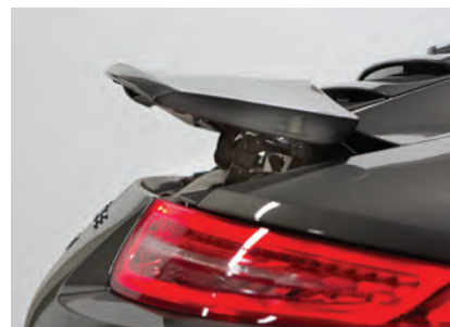
LIFT OFF The functional rear spoiler rises at 75 mph to increase down force. It retracts once the car has slowed to 45 mph.
