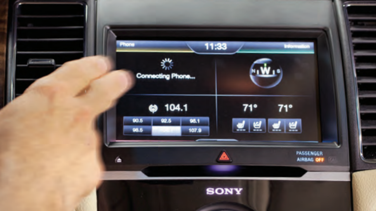
ELECTRONIC BUGS The MyFord Touch system suffered from unresponsive screens, freezes, and Bluetooth pairing problems.
