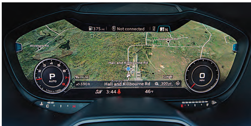
A NEW VISION Climate, map, and stereo displays are integrated into the instrument panel.
