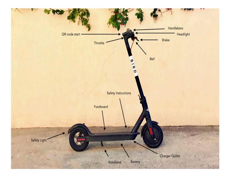
Our vehicle is completely electric and provides a comfortable yet efficient ride. With a top speed of 15 miles per hour, the Bird scooter will get the rider to their destination on time. The four-digit identification is located in between the handle bars.
